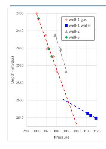
Wireline pressure data is often used to estimate the hydrocarbon-water contact. However, it can show a number of key reservoir characteristics:
