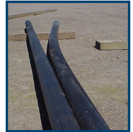
Drill Collars Bent Uni-Directionally
